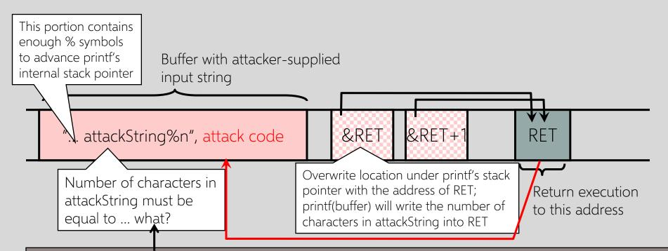
C has a concise way of printing multiple symbols: %Mx will print exactly 4M bytes (taking them from the stack). Attack string should contain enough "%Mx" so that the number of characters printed is equal to the most significant byte of the address of the attack code.
